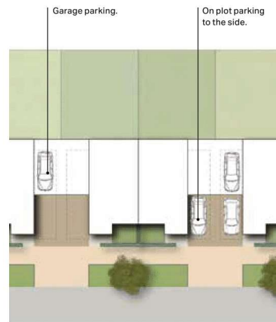
Double garage parking (and on plot parking to the side).
